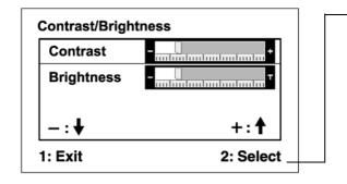
The command line at the bottom of the control screen tells what to do next from this screen. You can toggle between control screens, adjust the selected option, or exit the screen.
